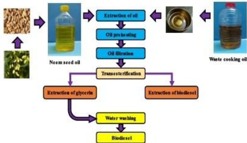
Fig. 1. Transesterification Process for Biodiesel Production
